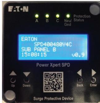
To enter the main menu from the home screen, push the enter key. The following selections will then appear on the screen. The less than symbol "<" represents the cursor location and will appear to the right of the selected menu category. Press the down arrow to scroll down through the selections or press the up arrow to move up. Press the enter button to select a menu item or press the back button to return to the previous menu screen.
