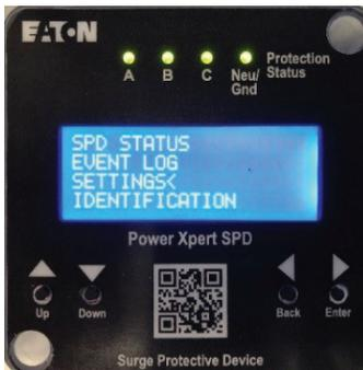
3. Enter a 6-digit password by pressing the Up button to the desired first number, if you go past the number press the Down button. Then press Enter to go to the next digit. Repeat the process until all six digits have been entered. After all six digits have been entered press Enter to continue.
