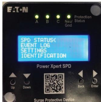
2. Scroll down the menu to settings by pressing the down arrow button. The cursor "<" is located to the right of the menu category selection. Position the cursor to the right of settings< by pressing the Down button twice and then press Enter.
