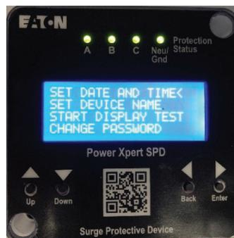
5. Press the Enter button to edit the date and time or the back button to exit and return to the previous screen.
