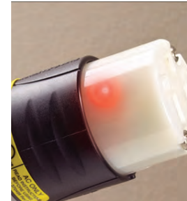
RED LED Open ground or reversed polarity
