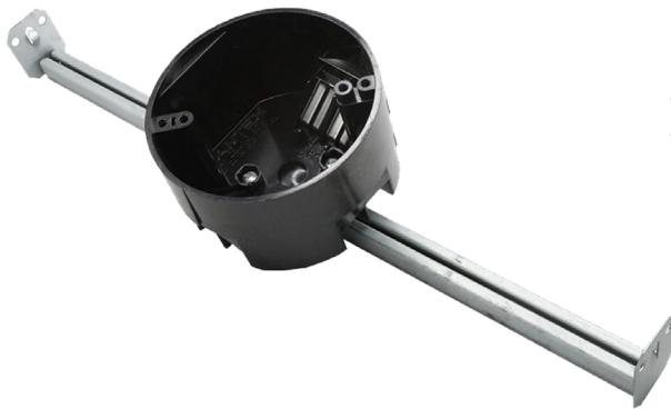
EZ20CHL EZ BOX is a 20 cu. in., new work (new construction) ceiling box with an attached bar hanger for adjustable, support between ceiling joists. EZ20CHL is for residential and light commercial ceiling applications. EZ20CHL features 6 wire clamps and an adjustable bar hanger that adjusts from 14" to 24" for added support and installation options.
