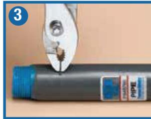
In **Step 3**, the tab is pulled perpendicular to the conduit with a pair of pliers. The plastic tab will tear off rather than having any peeling effect or the coating separating from the substrate.
