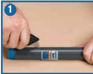
**Step 1** consists of two cuts through the plastic to the substrate along the length of the conduit, approximately ½" apart and 3" to 4" in length. A third, perpendicular cut crosses the lengthwise parallel cuts.
