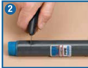
**Step 2** calls for the edge of the PVC that was cut on the perpendicular to be carefully lifted to form a plastic tab.
