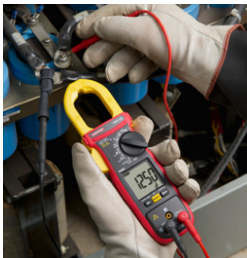
AMP-320 AC/DC Clamp Meter Electrical Motor Maintenance
