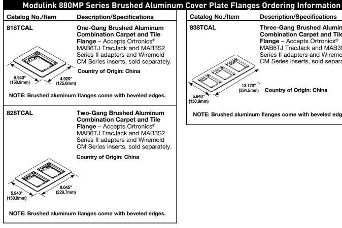
NOTE: Brass covers and flanges are not interchangeable with aluminum or nonmetallic covers and flanges. Nonmetallic covers are interchangeable with aluminum flanges.
