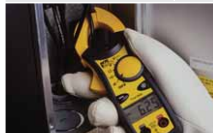
Compact jaw for use in tight locations
