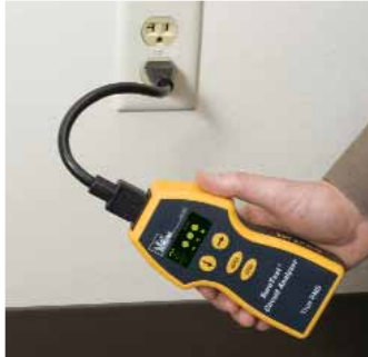
Troubleshoots branch circuit problems with a variety of tests at the receptacle.
