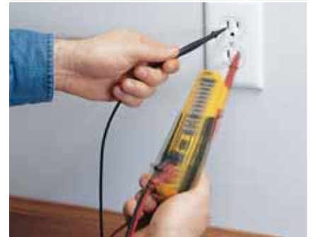
Vibration mode gives a tactile indication of the voltage level.
