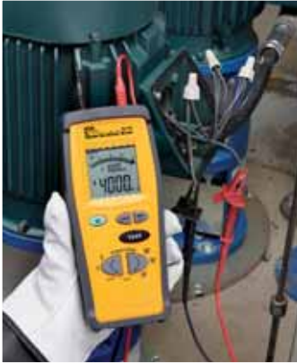
Tests insulation on motor windings
