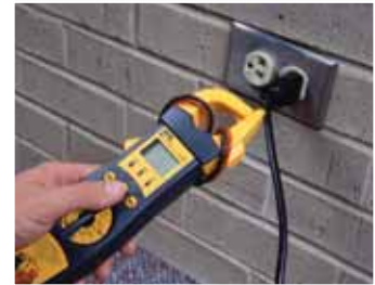
2: Non-Contact Voltage Tester Use it for one-touch indication of power without test leads.
