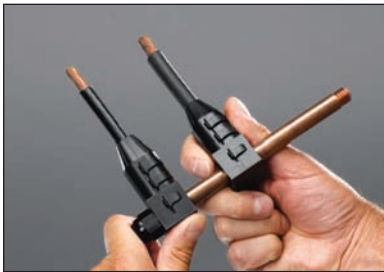
4. Slide connector/insulator assemblies onto rod.
