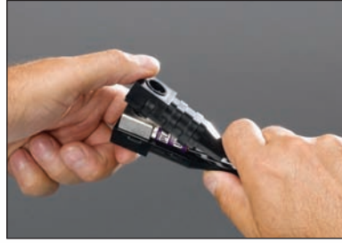
2. Snap Multi-Tap insulators over connectors.
