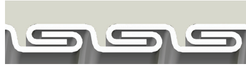
Interlocked Design 1-1/2" through 4" with no bonding wire
