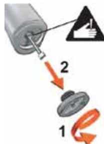
Storage Compartment for an extra blade (P/N 10018C sold separately).
